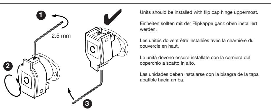
Units should be installed with flip cap hinge uppermost.
