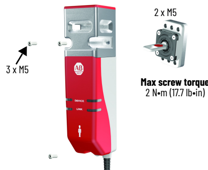
Figure 4 - Required Mounting Hardware for Switch and Actuator
